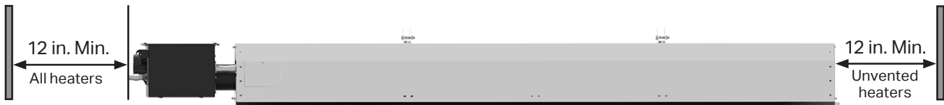
Figure 3.7 • Minimum End Clearances
